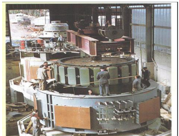
Fig 8. Rotor of a salient pole alternator
