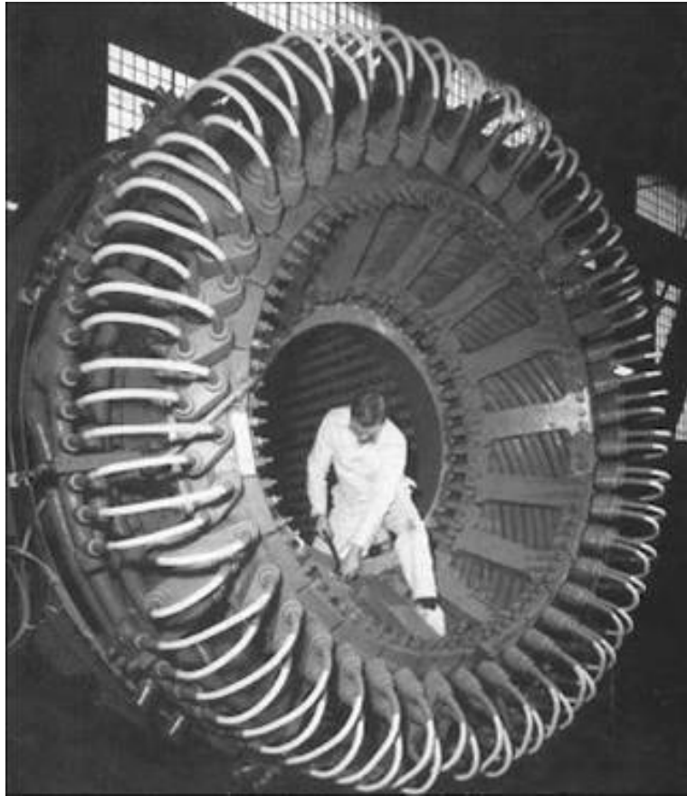
Fig 7. (a) Stator of a salient pole alternator
