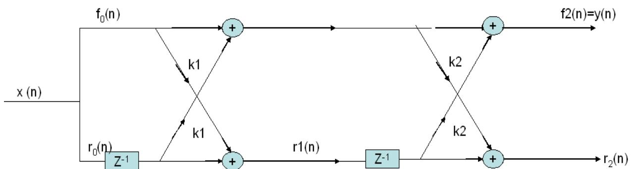
Similar to above, an  $M$ th order FIR filter can be implemented by lattice structures with  $M - 1$  stages
