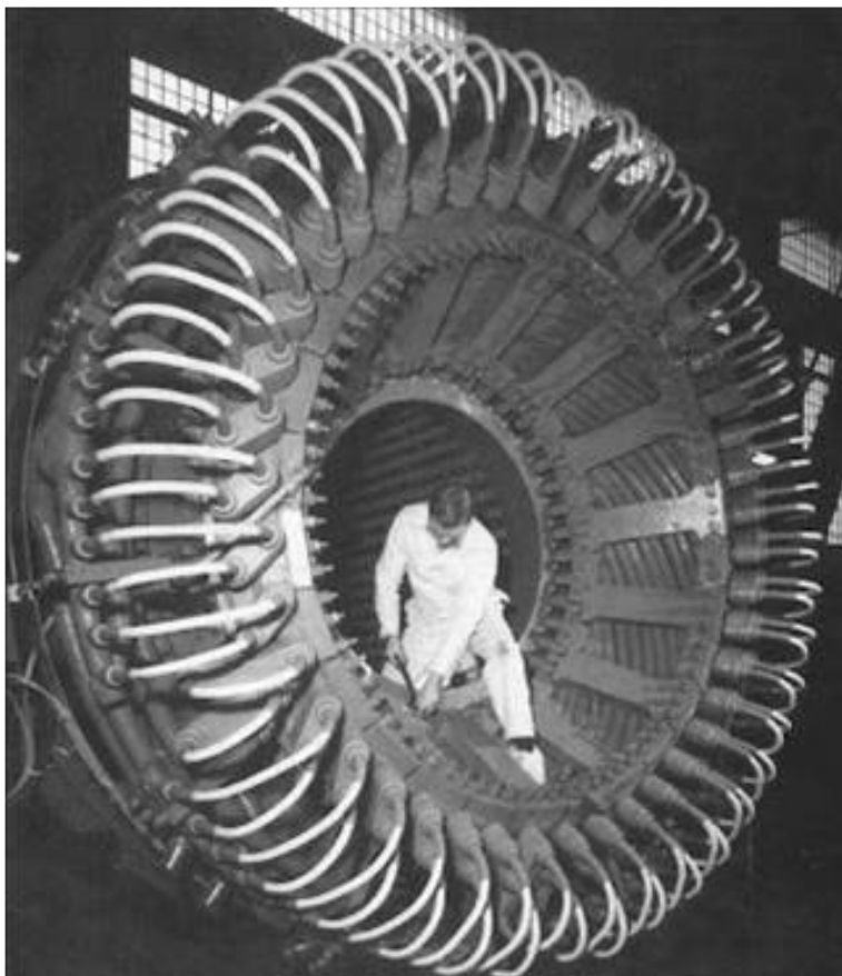
Fig 3. (a) Stator of a salient pole alternator
