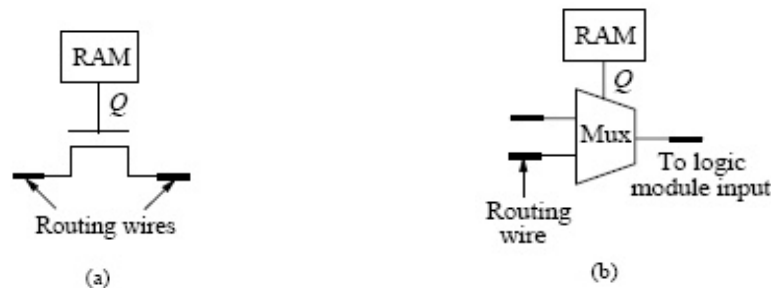
Figure 1.10: The SRAM Programming Technology. (a) A pass-transistor switch. (b) A multiplexer switch
